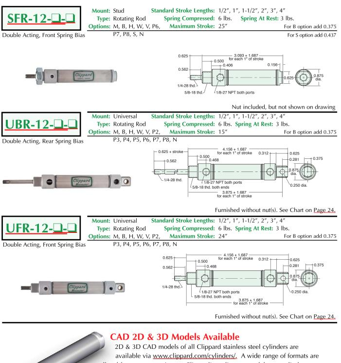
offered for your convenience. Clippard's on-line, state-of-the-art cylinder configurator allows users to build their own cylinder exactly to the required specifications, and then view the details, drawings, CAD models, pricing and much more! www.clippard.com/cylinders/
